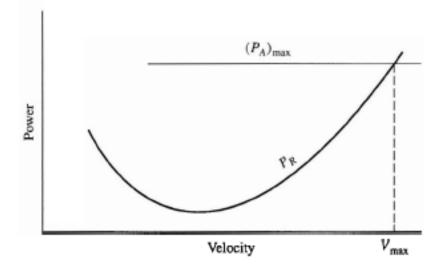
For a propeller driven airplane, the power available **PA** is essentially constant with velocity. The intersection of the maximum power available curve and the power required curve defines the maximum velocity for straight and level flight
