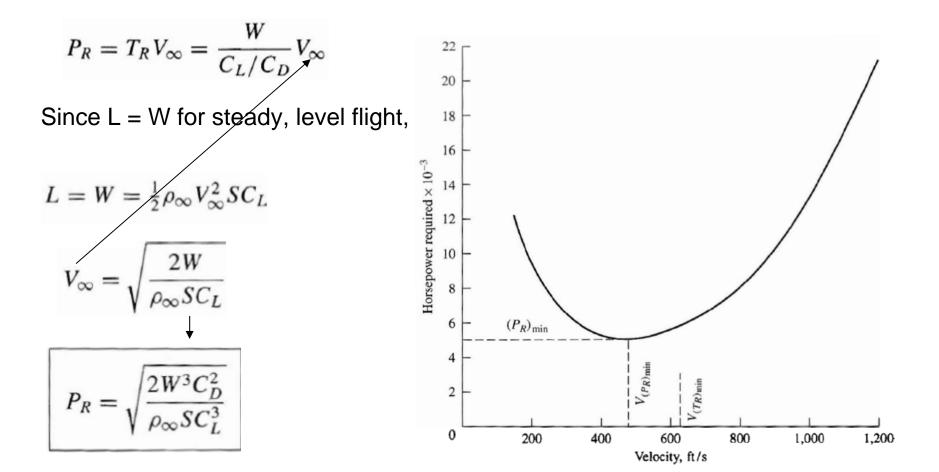
The minimum power required occurs when the airplane is flying such that  $\frac{C_L^{3/2}}{C_P}$  is maximum. By replacing *CD* with the drag polar, this expression can be written as
