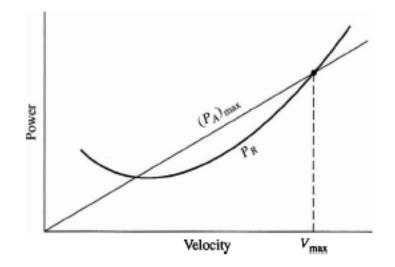
For a turbojet-powered airplane, assuming **TA** is constant with velocity, the power available at subsonic speeds varies linearly with V. The high-speed intersection of the maximum power available curve and the power required curve defines the maximum velocity for straight and level flight.
