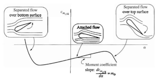
over most of the practical range of the angle of attack the slope of the moment coefficient curve is essentially constant.
