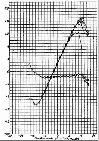
The slope of this linear portion is called the lift slope and is designated by a0. For thin airfoils, a theoretical vature for the lift slope is 2pi per radiant, or 0.11 per degree.
