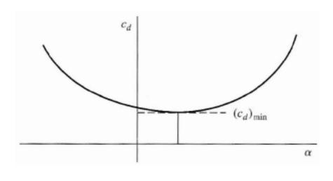
For a cambered airfoil, the minimum value cd does not necessarily occur at zero angle of attack, but rather at some finite but small angle of attack. For this angle-of-attack range, the drag is due to friction drag and pressure drag. In contrast, the rapid increase in cd which occurs at higher values of alpha, is due to the increasing region of separated flow over the airfoil, which creates a large pressure drag.
