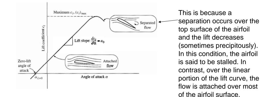
the linear portion of the lift curve is essentially insensitive to variations in Re. By increasing Reynolds number Clmax increases
