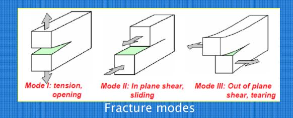
Stress intensity factor KIC can be described as fracture toughness of materials (material resistance to crack propagation) under conditions of :
