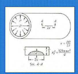
Flaw geometry and design of cylindrical pressure vessel
