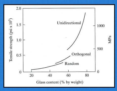
Effect of type, length, % volume, and orientation of fibers in a fiber reinforced plastic (nylon)
