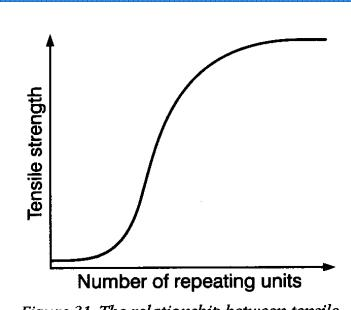
Figure 31 The relationship between tensile strength and chain length for a polymer.
