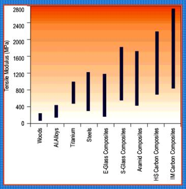
The lowest properties for each material are associated with simple manufacturing processes and material forms (e.g. spray lay-up glass fibre), and the higher properties are associated with higher technology manufacture (e.g. autoclave moulding of unidirectional glass fibre), the aerospace industry.
