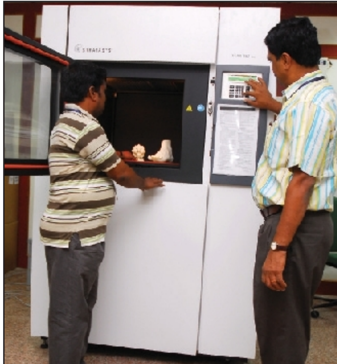
Left : The rapid prototyping machine; Top : Machine that calculates the dimensions; Below : 3 D models.
