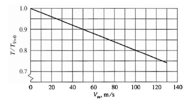
At higher subsonic velocities for a given, constant altitude, the decrease in thrust with Mach number can be correlated by T
