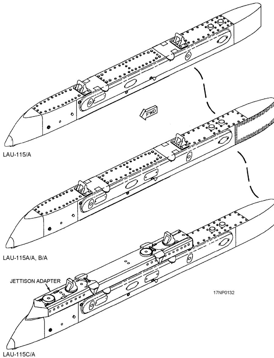
Figure 3-21.—LAU-115A/A, LAU-115B/A, and LAU-115C/A guided missile launchers.
