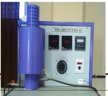
9. Thermal conductivity of metal rod
