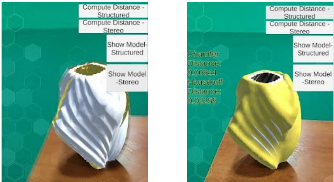
Fig 2: Real-world overlay showing CAD model + stereo/structured light scan with metrics.
