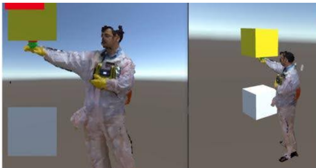
Figure 1 Virtual Clash Detection with Depth Camera.
