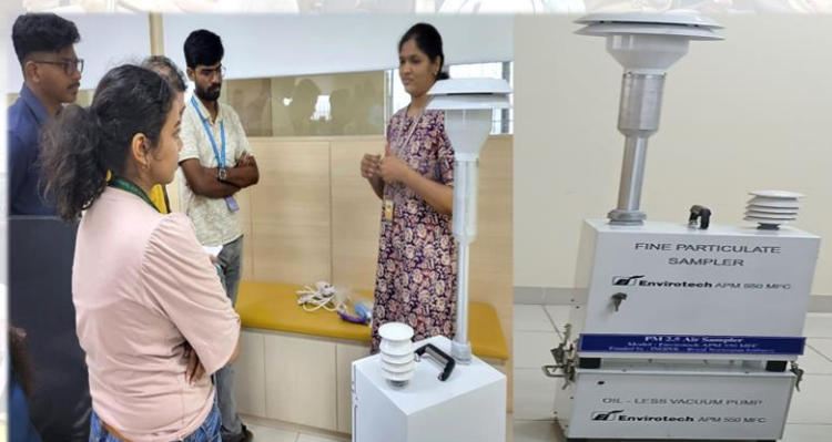
Demonstration of PM 2.5 air sampler
