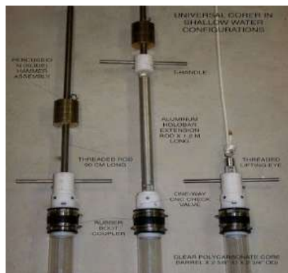
Figure 8.3: Sediment corer for core sampling
