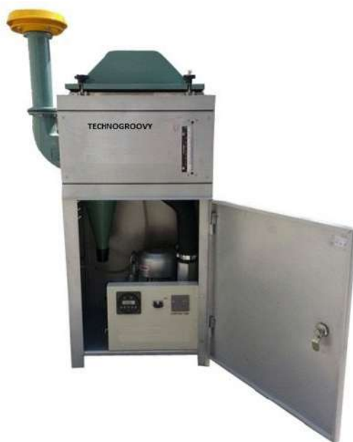
Figure 8.1: Typical high-volume air sampler
