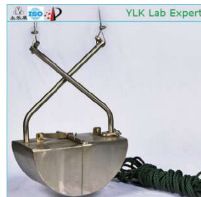
Figure 8.5: Grab sampler for sediment collection
