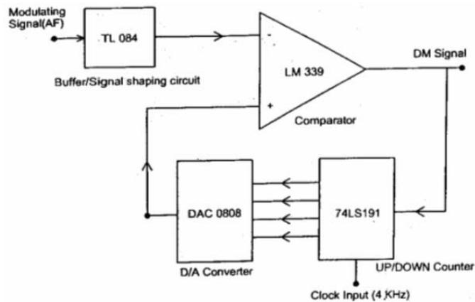
**Fig.4.1. DM Modulator**
