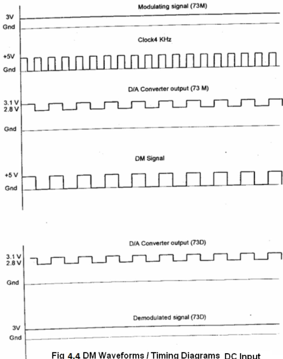
**Fig 4.4 DM Waveforms / Timing Diagrams DC Input**
