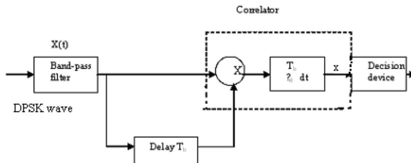
**Fig 12.2 DPSK Receiver Block Diagram**
