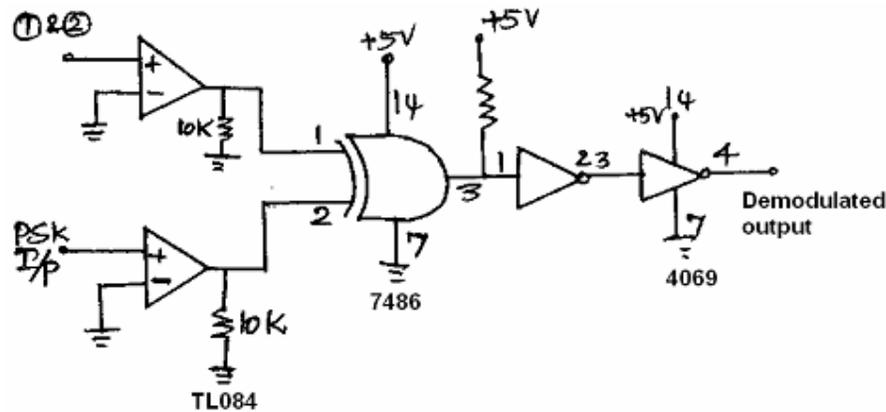
**Fig 6.3 PSK Demodulator**
