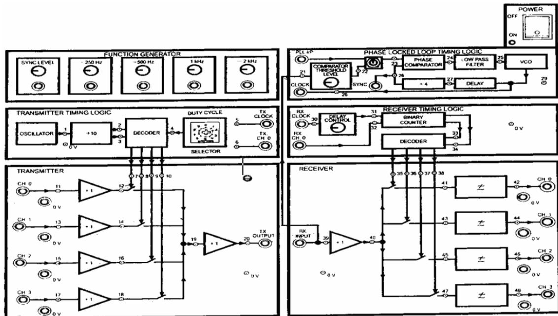
Figure 1.1 TDM Trainer Kit –ST2102 Block Diagram
