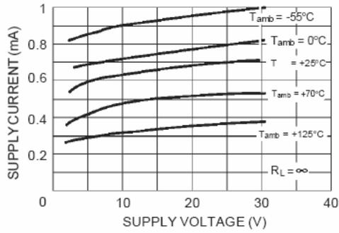
INPUT CURRENT versus SUPPLY VOLTAGE
