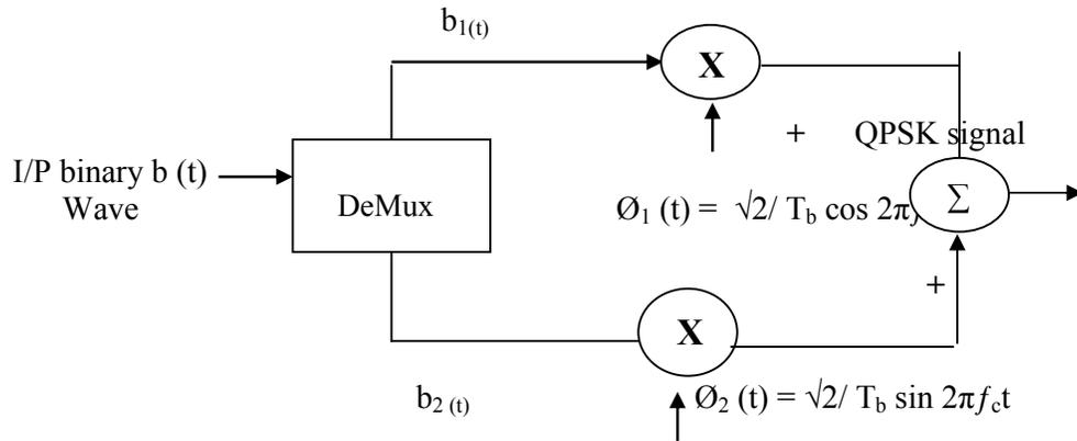
**Fig 11.1 QPSK Transmitter Block Diagram**
