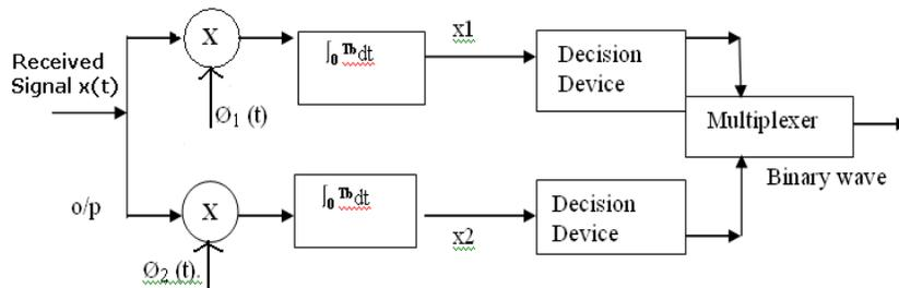
**Fig 11.2 QPSK Receiver Block Diagram**
