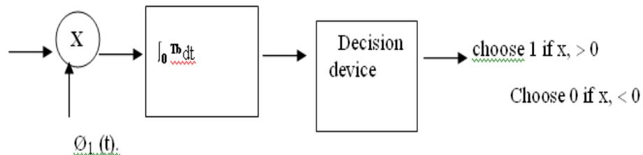
**Fig 8.2 ASK Receiver block diagram**
