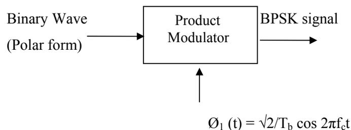
**Fig 10.1 PSK Transmitter Block Diagram**
