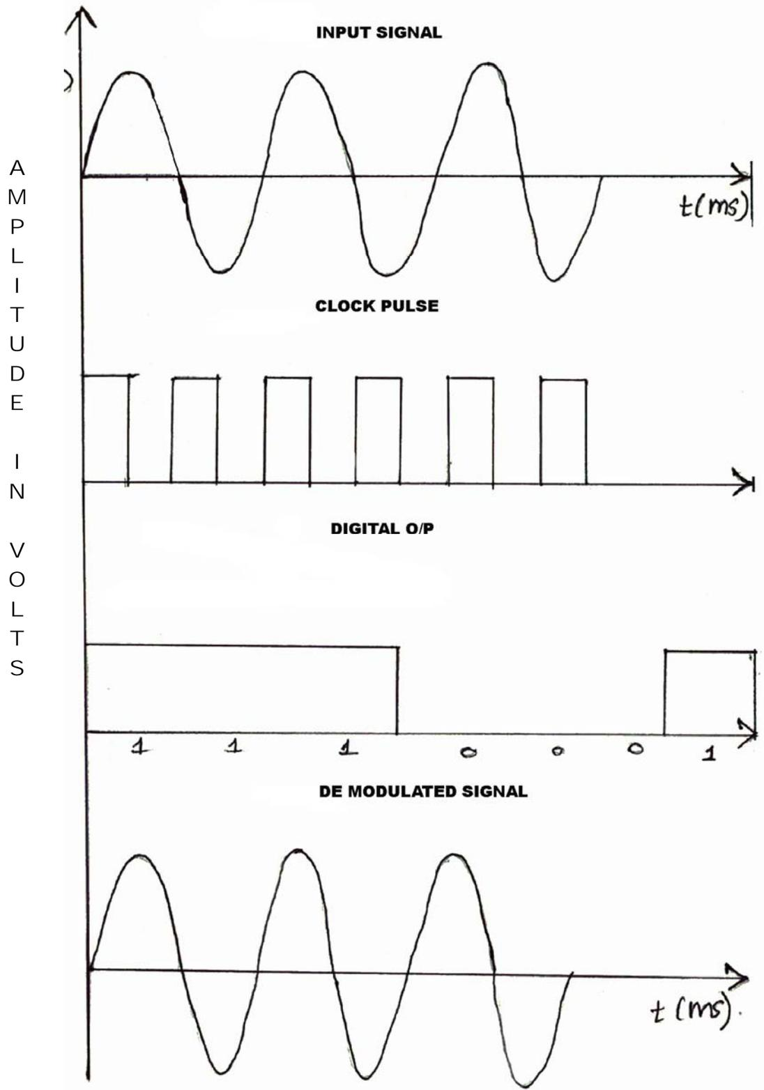
**Fig 2.2 PCM Waveform with AC input**
