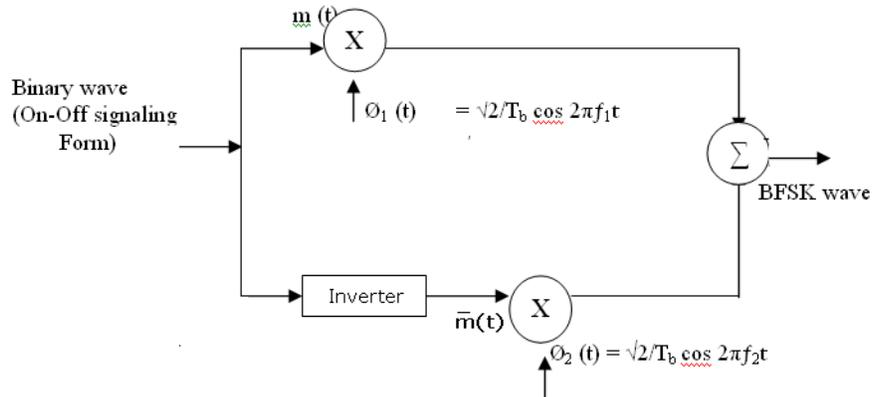
**Fig 9.1 FSK Transmitter Block Diagram**
