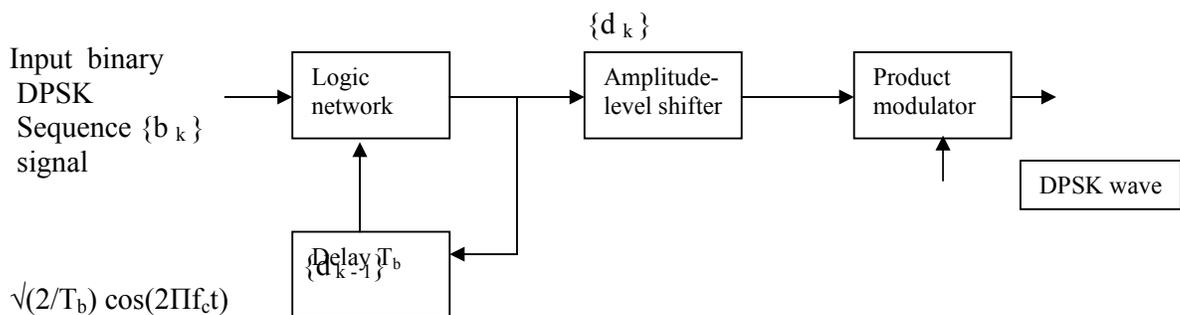
**Fig 12.1 DPSK Transmitter Block Diagram**
