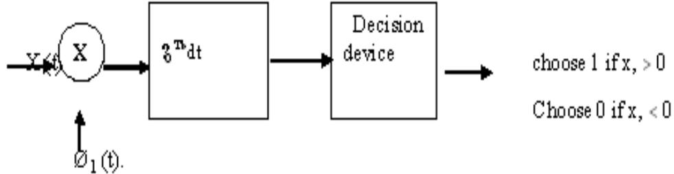
**Fig 10.2 PSK Receiver Block Diagram**
