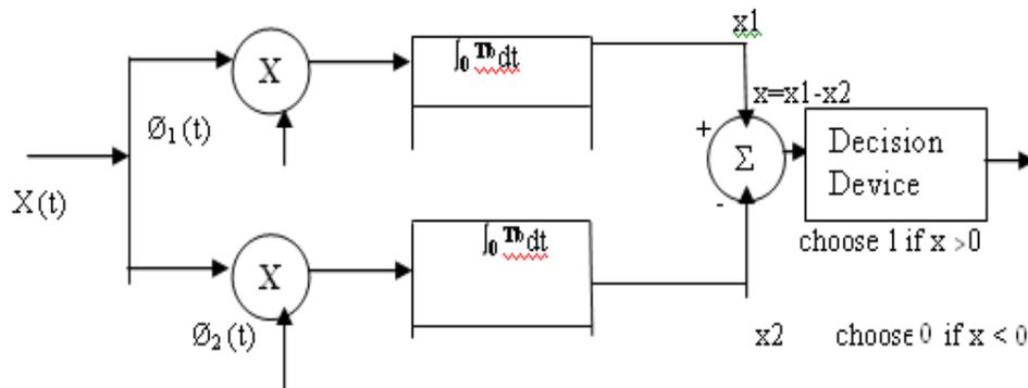
**Fig 9.2 FSK Receiver Block Diagram**
