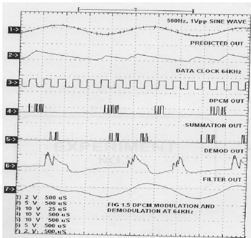
**Fig.3.2 DPCM OPERATION (with AC input) MODULATION & DEMODULATION**
