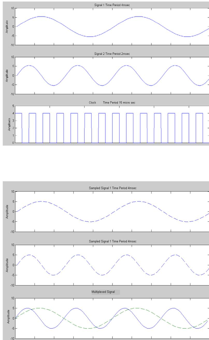
**Figure 1.2 TDM Multiplexed Signal**
