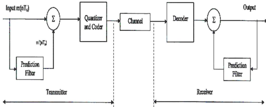
**Fig 3.1 Block diagram of DPCM System**
