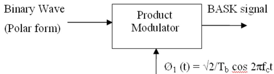
**Fig 8.1 ASK Transmitter block diagram**
