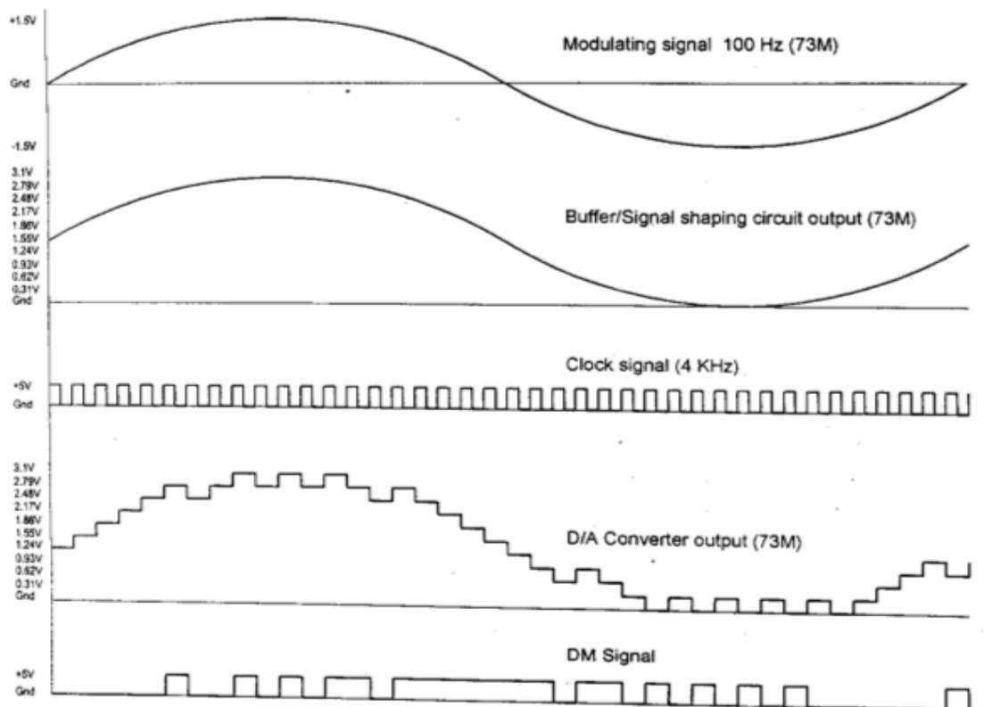
**Fig 4.3 DM Waveforms for AC input signal**
