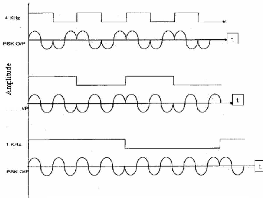
Fig 6.4. PSK Waveforms for different data input signals
