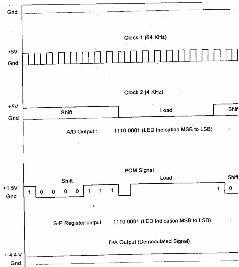
Fig 2.3 PCM Waveforms/Timing diagram(DC Input)
