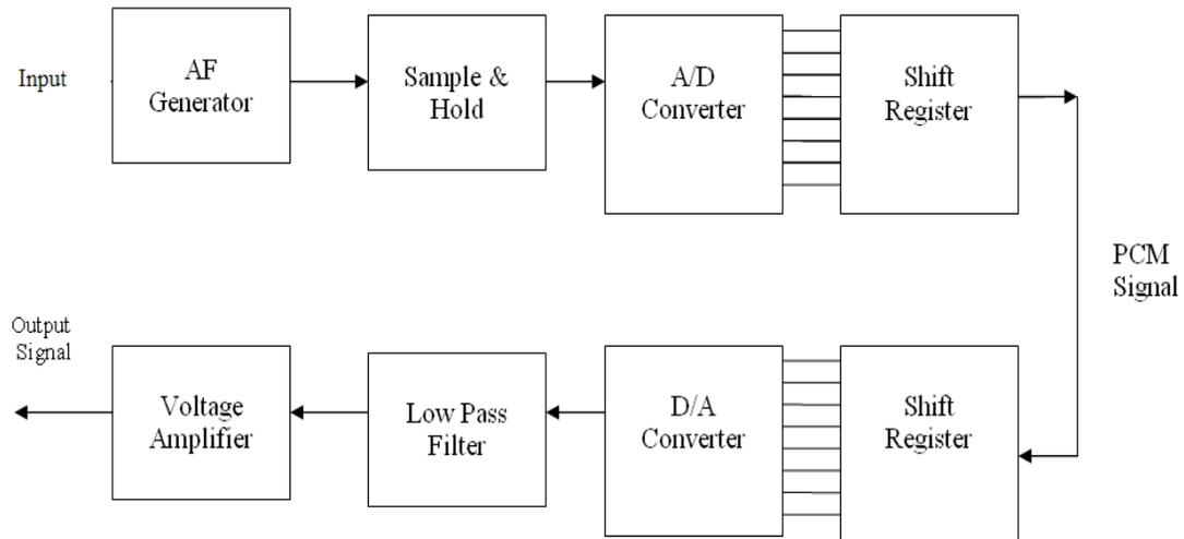
**Fig 2.1. PCM Modulator AND Demodulator**
