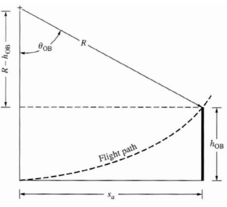
$$n = \frac{L}{W} = \frac{\frac{1}{2}\rho_{\infty}(1.15V_{\text{stall}})^2 S(0.9)(C_L)_{\text{max}}}{W}$$
