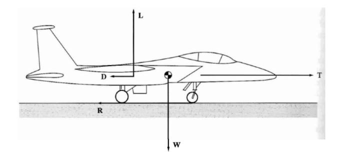
In addition to the familiar forces of thrust, weight, lift, and drag, there is a rolling resistance R, caused by friction between the tires and the ground.
