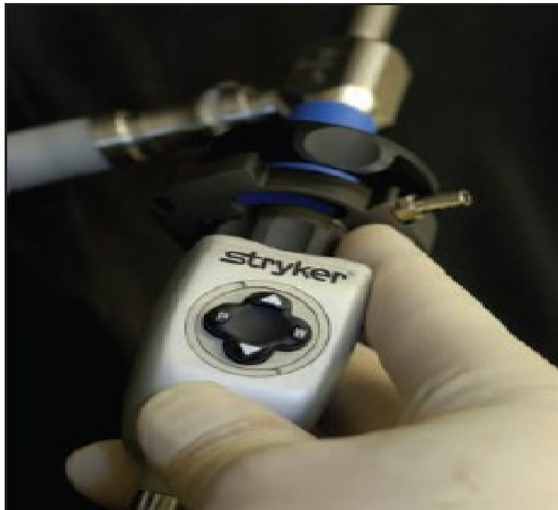
Figure 9. A three-chip camera attached to a laparoscope. Care should be taken to keep the camera upright (i.e., controls facing upward) at all times, even when the laparoscope is rotated to vary the field of view in the abdomen.
