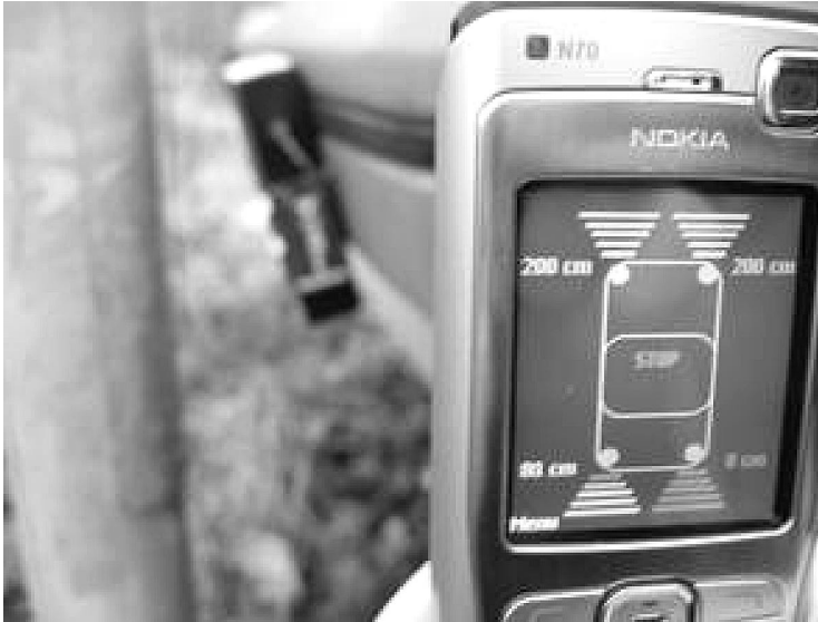
Figure 2.7 Parksensor with mobile phone application [15].
